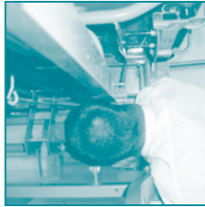
Bed frames should be checked to assure safety stops are in place to minimize crush risk to patients.
